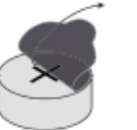
2. Pull the protective foil off the "+" side of the new battery.
