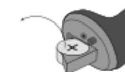
1. Open the battery compartment fully and remove the battery.
